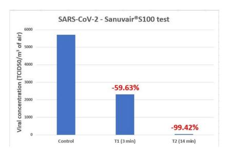
\* After 14 minutes, the Sanuvair® S100 unit has reduced the number of viable SARS-CoV2 viruses in the air by a factor of 200 times less.
